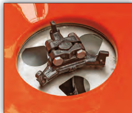
Agitator ensures even feed of the fertiliser
