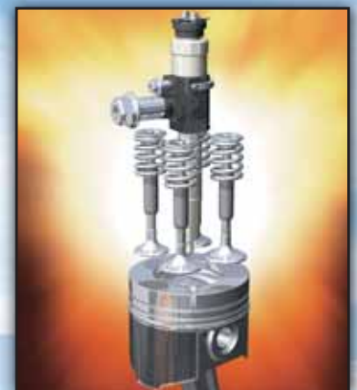
4-valve, Center-Direct Injection System
